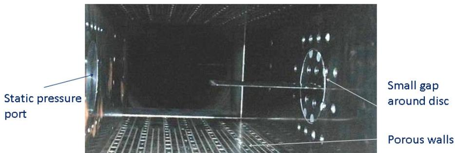
Figure 2: View upstream of Ludwieg tube showing the wall-mounted wing tip.
